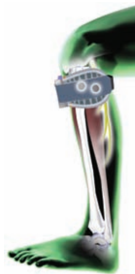
Figure 3: The WalkAide System Has the Unit and Cuff in a Single Component and Can Be Used Without Shoes
