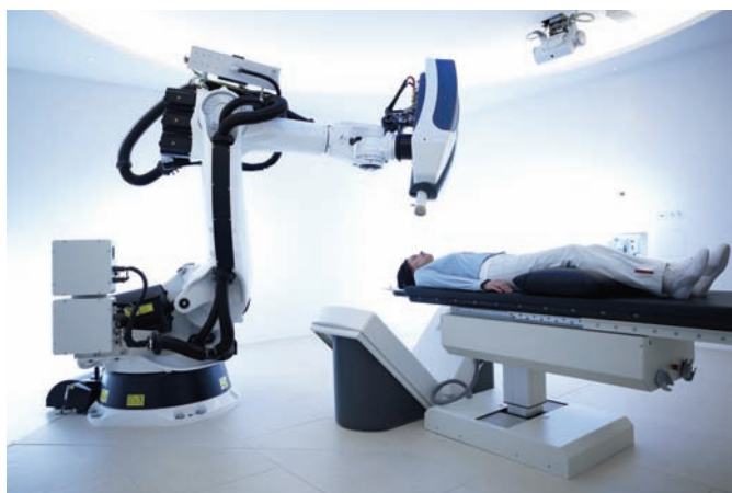
Figure 1: The Cyberknife System with Major Components Such as the Treatment Couch, X-ray Detectors (Silicon Detectors), X-ray Cameras at the Ceiling, Robot and Compact Linear Accelerators
