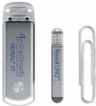
Figure 2: Reveal XT and the Recently Launched Reveal LINQ, Side by Side for Size Comparison
